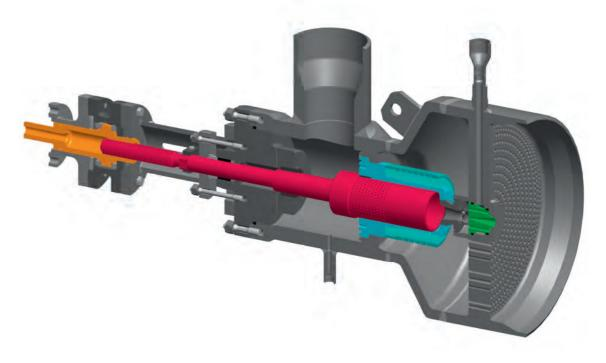
In the outlet of a steam converting station integrated steam-atomising desuperheater
