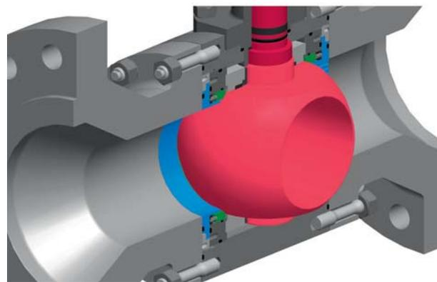
subcritical pressure reduction. Further-reaching requirements for a multi-stage pressure reduction can be achieved with additional fixed perforated discs. The ARTES control ball valve G is bi-directional and can thus be used as a supply or discharge control valve in natural gas storage or as a pressure control valve between different gas networks.
