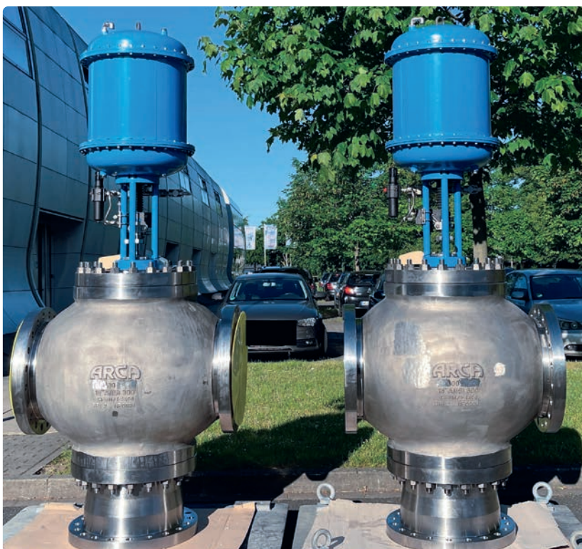
These two enormous 16" ANSI 300 3-way valves regulate the temperatures in the steel production of the new electro-steel plant in Sinton (Texas).
